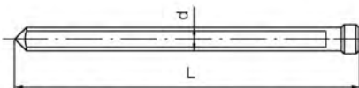
φ 8x90 适用于直径3/4"—2-1/2"mm的钢板钻 Suitable for diameter from 3/4" to 2-1/2"
