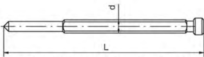
φ 6.35x90 适用于直径12mm—65mm的钢板钻 Suitable for diameter from 12mm to 65mm
