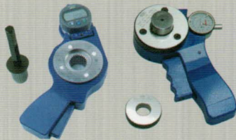
Handheld circular tooth thickness/space width gage with setting master
